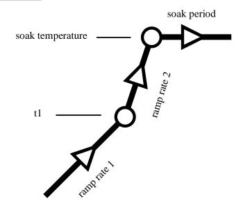
An ST316B firing segment comprises 2 ramps followed by a soak period. A single segment can be used for simple firing (biscuit firing for example) or up to 9 segments can be used per program for complex firing (crystal glazing or glass-making for example).
