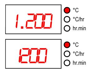
If the left-hand decimal point in the display is lit then the ST316B is locked. Press and hold in both the ♠ & ♣ keys for 5 seconds to unlock the ST316B.
