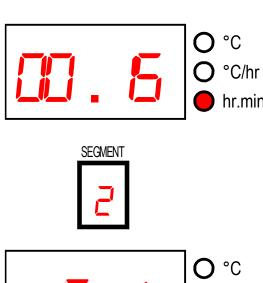
The next push of the → key displays the soak time in the range 00.00 to 99.59 (99 hours 59 mins). This can be altered with the ★ & ↓ keys. The SOAK TIME LAMP on the mimic display will flash.
