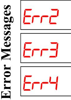
Error 2. Thermocouple or thermocouple wiring open circuit. Get thermocouple and wiring checked. Have thermocouple replaced if necessary.
